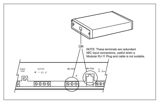
Figure 2-3. FM-14 Log Current Microphone
